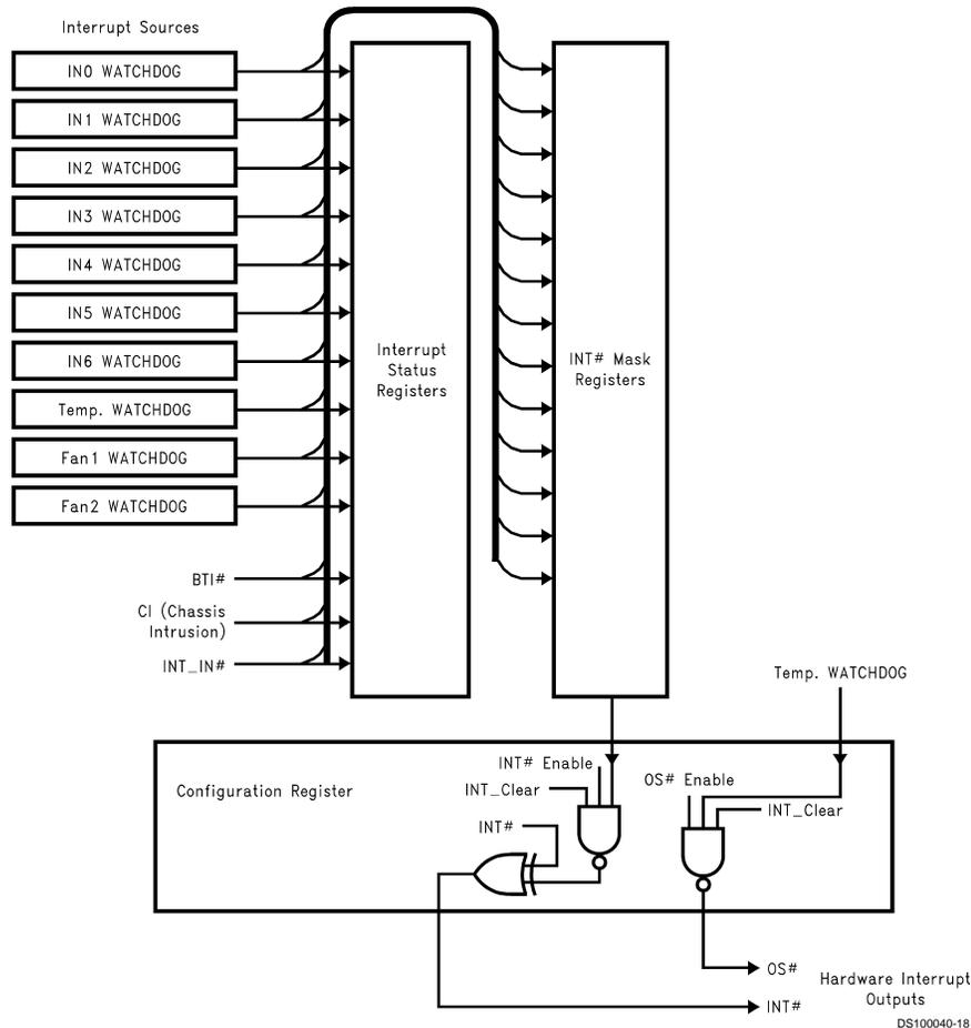
FIGURE 10. Interrupt Structure
